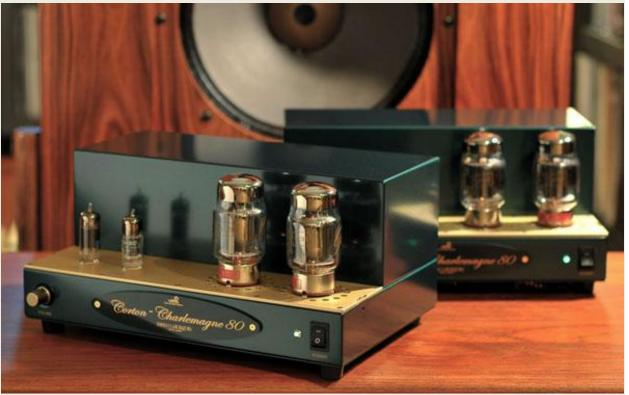
Ken Shindo's highest powered amplifier with 70 watts per channel into 8 ohms. Uses two KT88s per channel and manages to have the finesse of a single ended triode with the power to drive most reasonable loads.
